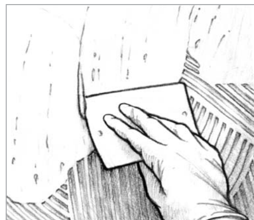
Figure 8 Trowel a second layer of fairing compound over the surface to fill the grooves after the ridges have been sanded fair.
